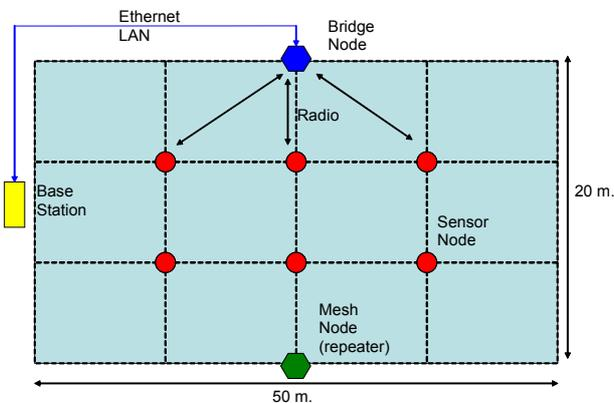
**Figure 2. Sensors field structure for the experiment**
